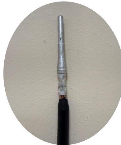
Crimp at \frac{1}{4} " from the edge Rotate 90 deg. Crimp \frac{1}{4} " from first crimp
